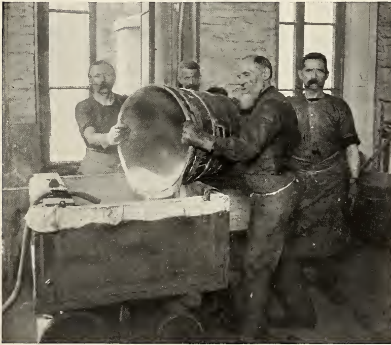
WASHING THE GOLD "MUD" WITH HOT WATER PREPARATORY TO PRESSING INTO CAKES.
